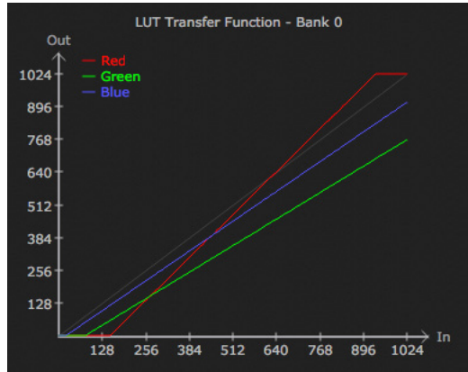
Figure 15. Example LUT Transfer Function Curves
