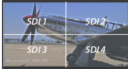
Figure 7. Mapping of Quad SDI Outputs
